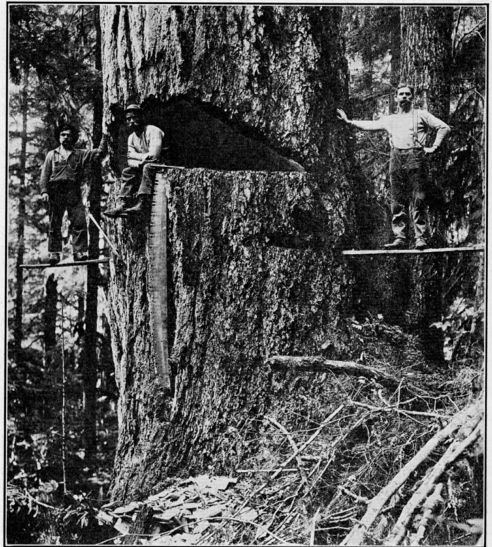
FIG. 47.—Undercut on a large sized Douglas fir tree in the Pacific Northwest. Spring-boards are generally used to get above the debris, fallen timber, etc., especially on steep hillsides. These spring-boards are 2 by 8 and 3 by 8 inch boards with a sharp tongue screwed into the end and placed in notches. It may require several hours to fell a single tree of this large size.
