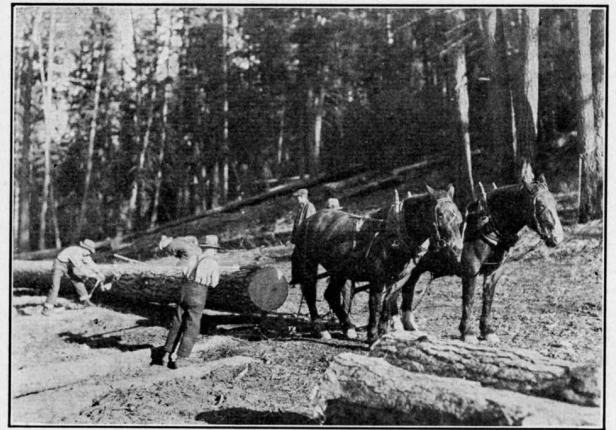
FIG. 39.—Bucking ponderosa pine logs at the landing. Long lengths are hauled to the landing by horse team or tractor, then bucked to shorter lengths to facilitate log loading and haul to the mill.
